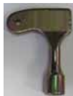
Figure 4: Auto Slim Landing Doors Emergency Opening
